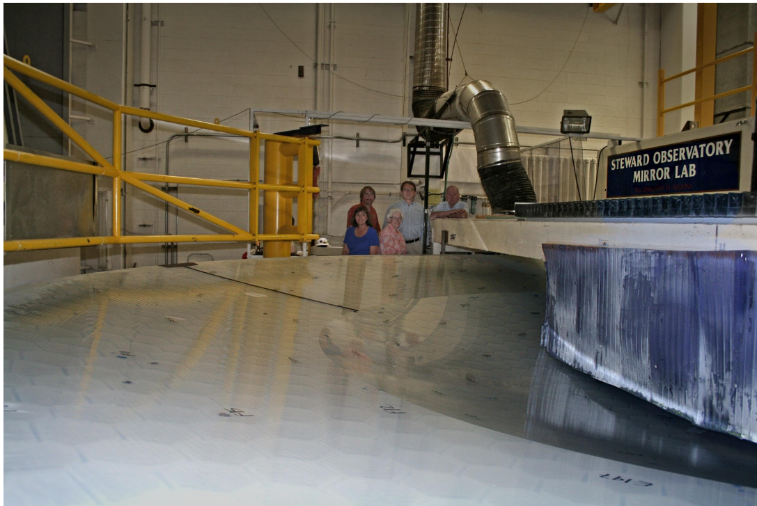
Grinding the 8.3m lens (Steward Observatory, Tucson, AZ)
