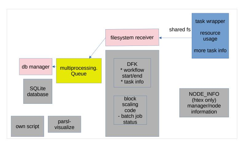
so the other option, which most executors have used by default in recent years, is the filesystem radio. That uses a shared filesystem directory: messages are written to the filesystem by the sender, and read out of the directory and fed into the queue by a receiver process.
