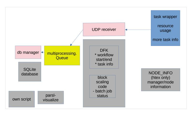
From the task wrapper, which is potentially running far away - the radio mechanism is pluggable. That's something I've worked on in the last year, with the intention that you can swap in different mechanisms here.
