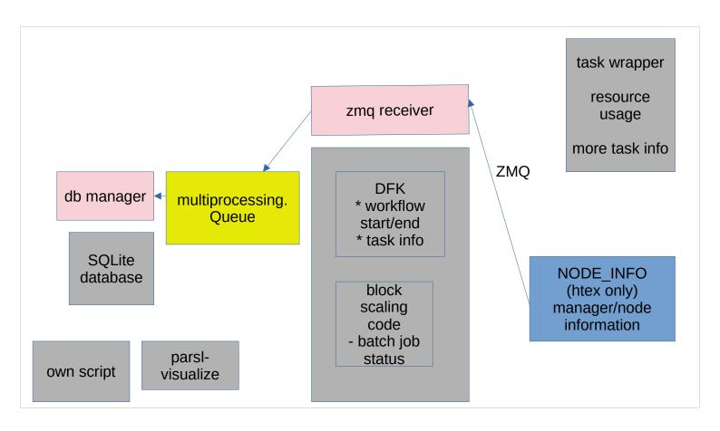
what about the other processes that aren't in the multiprocessing group? the processes running as task wrappers aren't even on the same computer - they're on worker nodes. so there's going to have to be some kind of networking involved. and the interchange is a completely separate unix process (for historical reasons) even though its on the same host.
