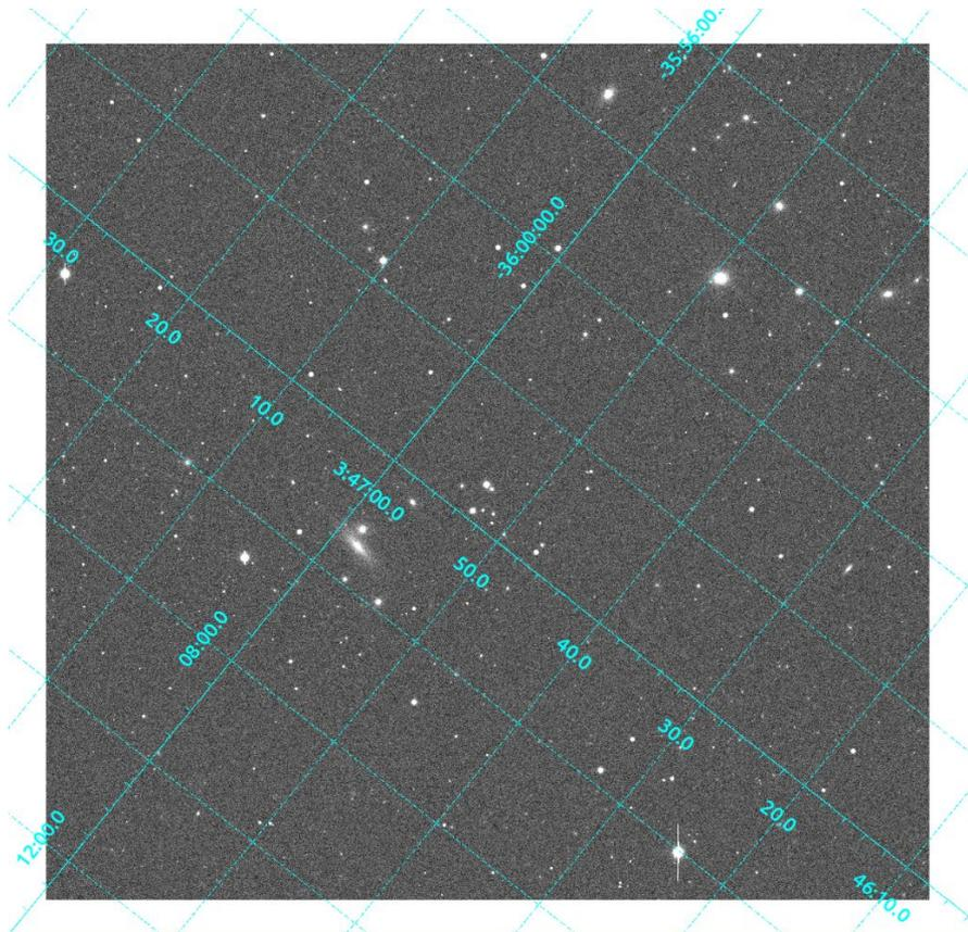
Raw CCD image for a single DC2 i-band 30s visit. Visit-level processing removes instrumental effects and performs the initial astrometric and photometric calibration.
